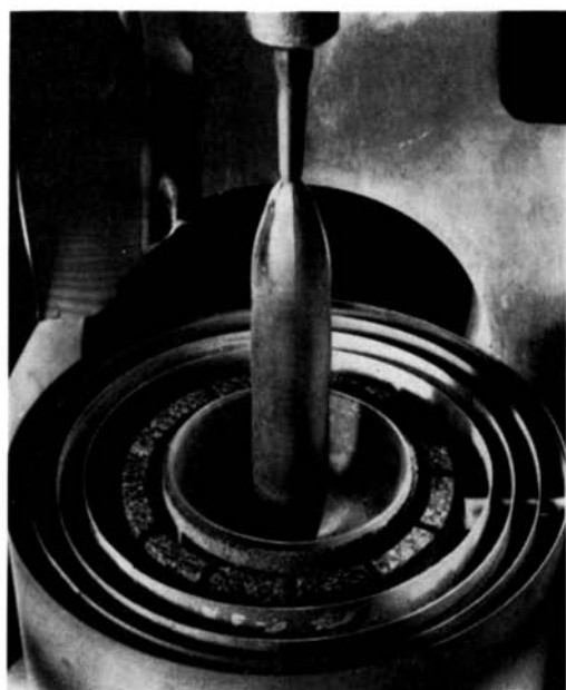
Figure 4.18. Improved Czochralski crystal pulling furnace; a) graphite heater; b) crystal, crucible, heater, and radiation shields. After Marshall and Wickham. 67 (Courtesy Services Electronic Research Laboratory, Baldock, Herts, England.)
