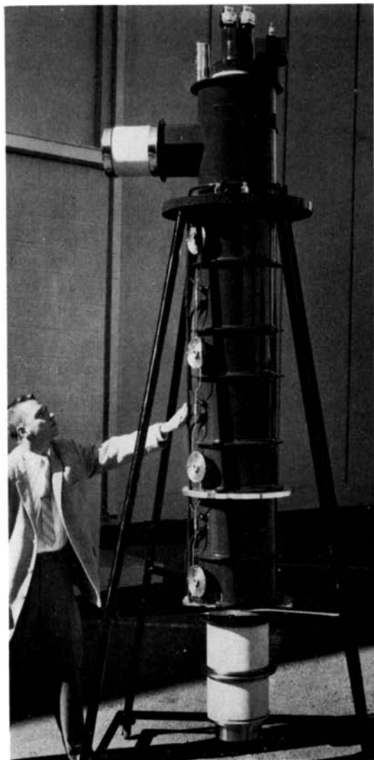
Figure 14.3(f). Type VA-842 Klystron; average power output 75KW, peak power output 1.25MW. Pulse duration 2 milliseconds, tunable frequency range 400-450MC, stable R.F. power gain 40db. (Courtesy Varian Associates.)
