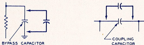
Fig. 2. On difficult service jobs it is a good practice to check all of the bypass and coupling capacitors in the suspected section of the receiver for possibility of open circuit: Temporarily connect a good capacitor across each of the suspected capacitors in turn. If connection of the good capacitor restores normal operation it may be assumed that the original capacitor is opened.
