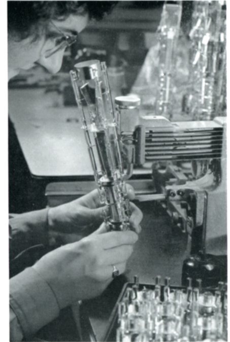
Assembling electrodes for five-inch tubes.
