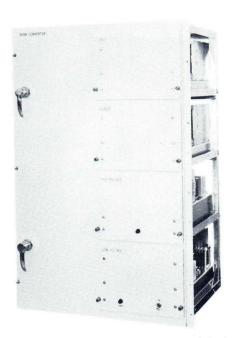
This completely transistorized scan converter converts x-y coordinates to PPI polar coordinates with a high degree of precision. The simulator accepts computer data and radar information and generates a simulated PPI scan.
