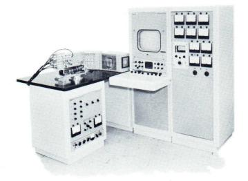
This equipment has been designed for rapid, complete, and accurate testings of vidicon tubes. Provisions can be included for automatic measurement of spectral response.
