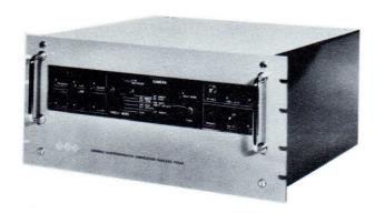
This completely transistorized test set is designed to provide a standard "Indian Head" test pattern over a wide range of slow scan frequencies with a rectilinear format. A 2F21 monoscope tube is used as the source of the video signal. Driving the DC coupled sweep amplifiers externally, any desired scanning program can be obtained. Sweep and blanking outputs are supplied with the video signal.
