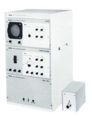
This completely transistorized TV system consists of camera head, camera control, monitor and power supply. The system provides continuously variable control of the scanning frequencies over a range of 100:1. It is capable of being modified to any specific slow scan or standard TV requirements. When used with the ED 6021 Scan Converter, the system provides complete slow scan operation for narrow band
