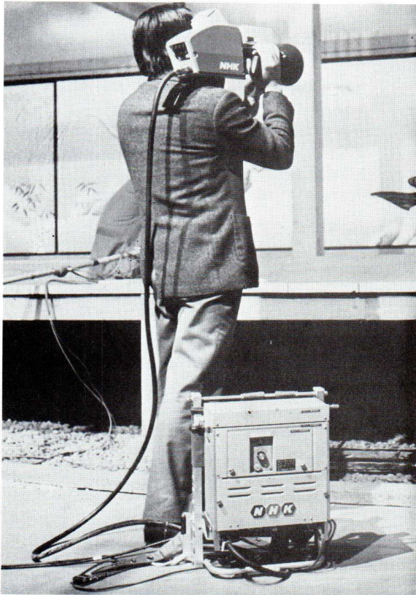
Photo 2. Broadcast Use Hand Held Camera Equipped with SATICON
