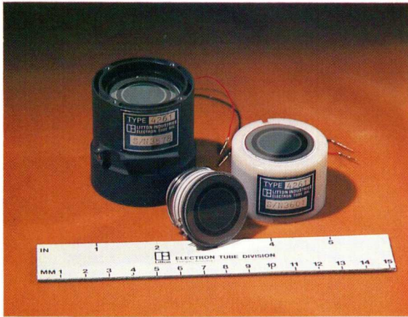
18mm image intensifier tubes; bare tube, tube with power supply, tube/power supply in metal housing.
