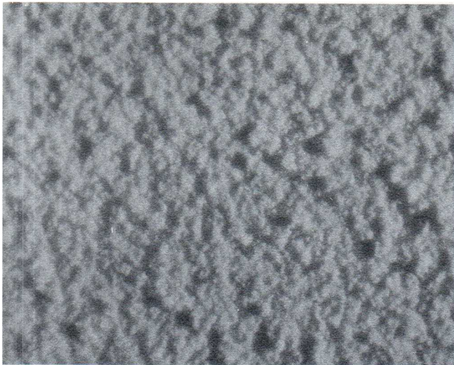
Figure 2 — Top view of standard cathode and Phormat cathode, right, shows porosity of Phormat surface. Porous matrix improves high voltage stability because it inhibits arc development. (Same magnification used for both views).
