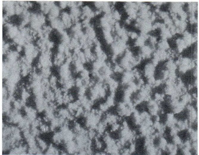
Figure 2 — Top view of standard cathode and Phormat cathode, right, shows porosity of Phormat surface. Porous matrix improves high voltage stability because it inhibits arc development. (Same magnification used for both views).
