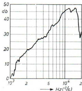
Fig. 82. Electrostatic speaker: a) Sound-pressure curve b) Radiation pattern at 12,000 c/s
