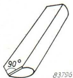
Fig. 13. The cutting stylus
