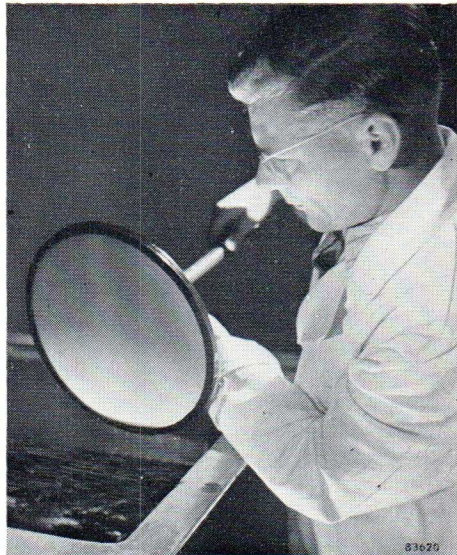
Fig. 14 Making a "father" in a plating bath
