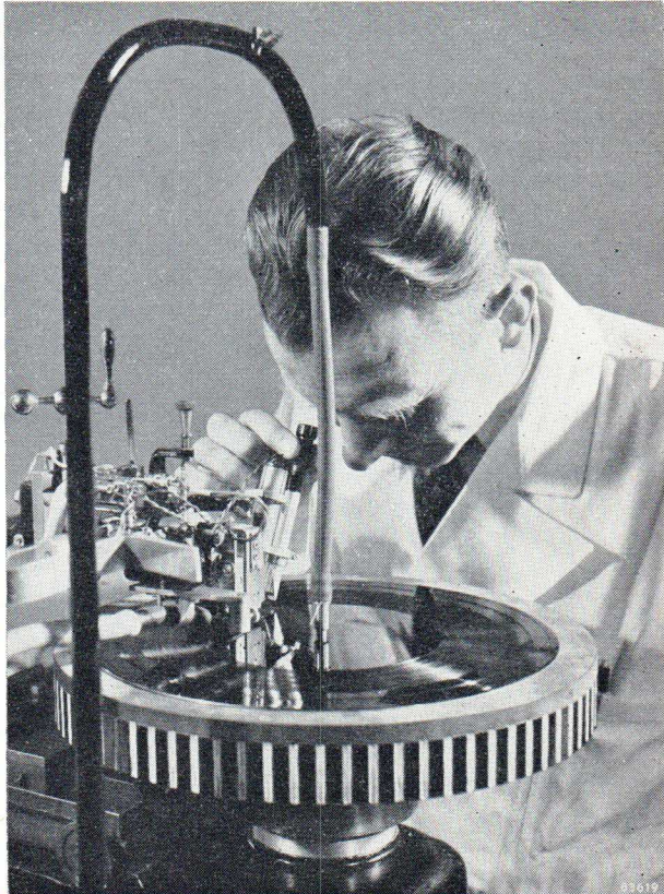
Fig. 12 Cutting the lacquer plate
