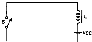
Fig. 85—Simplest form of deflection circuit.
