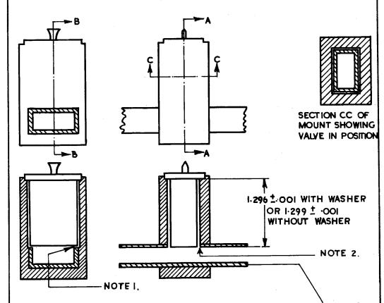
SECTION AA OF MOUNT SHOWING VALVE IN POSITION. SECTION BB OF MOUNT SHOWING VALVE IN POSITION. PIECE OF STRAIGHT WAVEGUIDE OF INTERNAL DIMENSIONS 0.4 BY 0.9.
