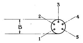
BULB STRAIGHTNESS. The finished valve must pass through a cylindrical gauge of length at least equal to that of the bulb. I.D. of cylinder = 0.218 inch.
