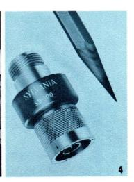
1/ Development of ferrite devices to accommodate new systems requirements are under way. An example is a high power broadband isolator capable of handling 2 Kw of average power and 20 Kw of peak power over a frequency band of 7.5 to 10.5 Gc. This unit is effective at temperatures up to 250°C and will handle in excess of 100 watts of reflected power with only convection cooling.
