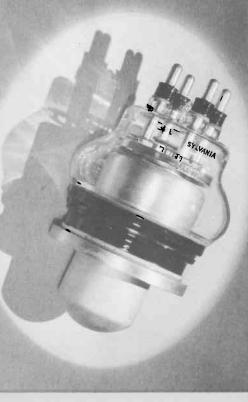
Forced-air-cooled coaxial-terminal triode for industrial heating service and AM broadcasting. Incorporates lightweight aluminum disc-finned anode cooler; rugged coaxial mounting structures, provide high-dissipation, low-inductance r-f electrode terminals. Heavy-wall anode. Thoriated-tungsten stress-free filament.
