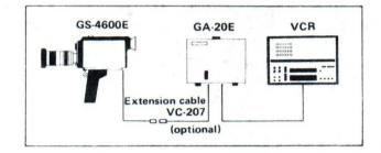
If the RF Converter is installed in the GA-20E and the GA-20E RF OUT jack is connected to the TV antenna terminal, the picture and sound can be monitored by setting the TV channel to that of the RF converter.
