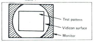
Zoom the camera lens until the resolution pattern as large as possible so that the pattern is not distorted. Keeping the camera and lens in this condition, adjust R69 (H. size) and R95 (V. Height) again for a correct aspect ratio. i.e.: The wedges at top and bottom of the test pattern, also the wedges on the sides of the test pattern reach the vertical and horizontal raster limits.
