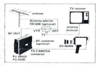
NOTE: When you only monitor the recorded tape on the TV receiver, you do not need to connect the camera to the VTR. Just set the TV-CAMERA switch to TV, and playback monitoring is possible using the VTR function lever.
