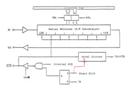
Fig. 2-3 The Block Diagram of Serial Ports
