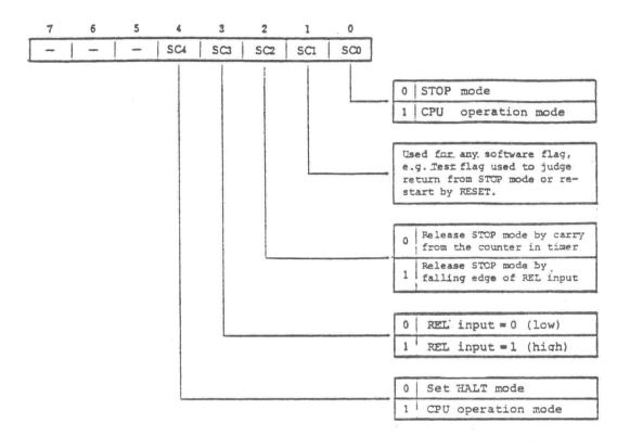
Fig. 2-9 Stand-by Control Register Format
