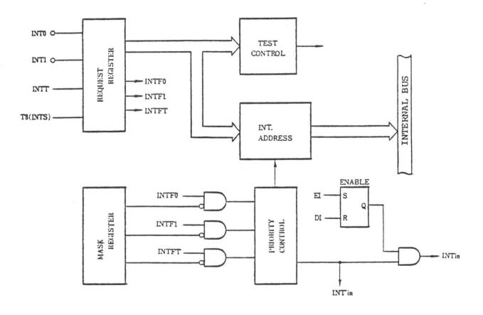
Fig. 2-10 Interrupt Control Block
