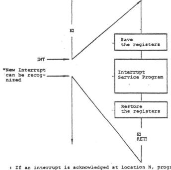
: If an interrupt is acknowledged at location N, program returns to location N after completing interrupt procedure.
