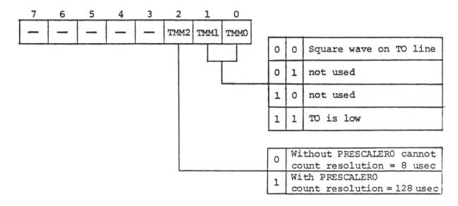
Fig. 2-6 Timer Mode Register Format
