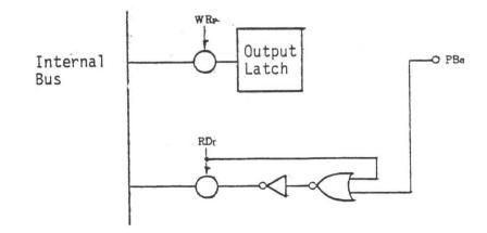
Fig. 1-2c The lines of the Port B used as input ports
