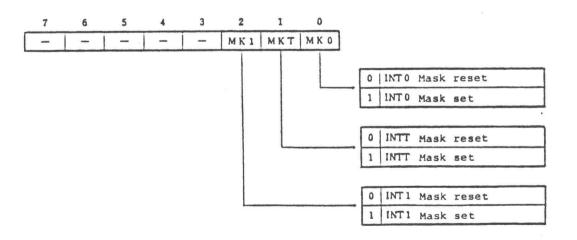
Fig. 2-11 Mask Register Format
