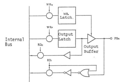
Fig. 1-2a The Port B Structure
