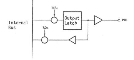
Fig. 1-2b The lines of the Port B used as output ports
