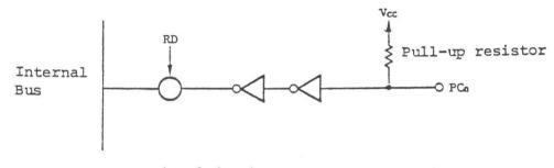
Fig. 1-3 The Port C Structure
