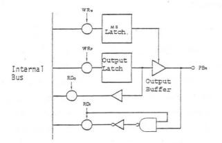
Fig. 1-2a The Port B Structure
