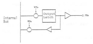
Fig. 1-2b The lines of the Port B used as output ports
