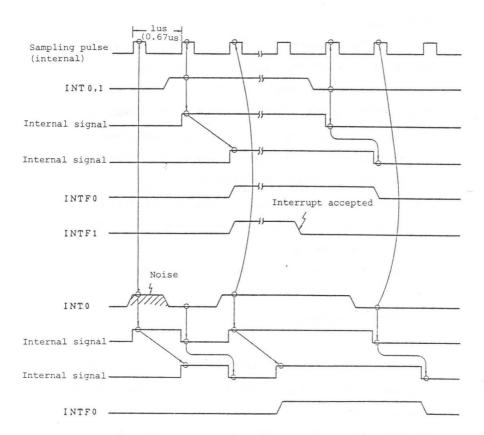
Fig. 3-2 Sampling of Interrupt
