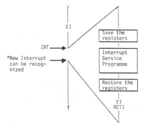
\*: If an interrupt is acknowledged at location N, programme returns to location N after completing interrupt procedure.
