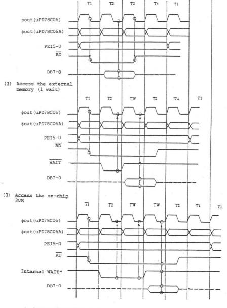
\* Two wait cycles are automatically inserted when the on-chip ROM access. 49
