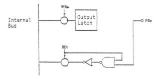
Fig. 1-2c The lines of the Port B used as input ports
