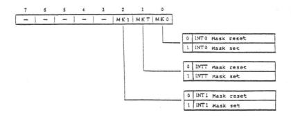
Fig. 2-11 Mask Register Format
