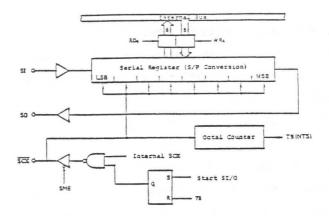
Fig.2-3 The Block Diagram of Serial Ports
