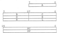
Fig. 2-1 Register Configuration
