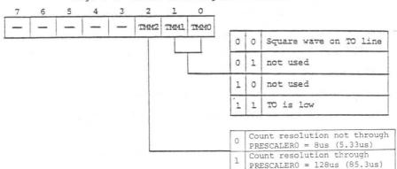
Fig. 2-6 Timer Mode Register Format
