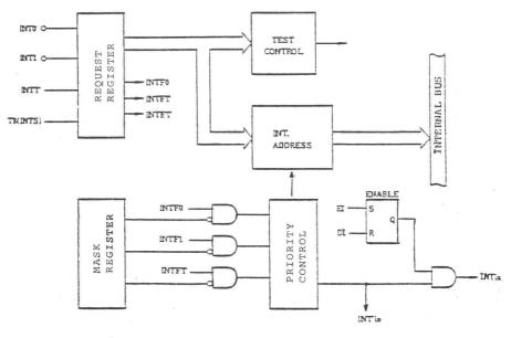
Fig. 2-10 Interrupt Control Block
