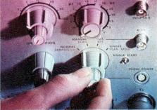
Front panel detail, above, shows clear layout of controls. Combination of circuit design, and ergonomy makes the PM 3400 as easy to operate as a real time oscilloscope.
