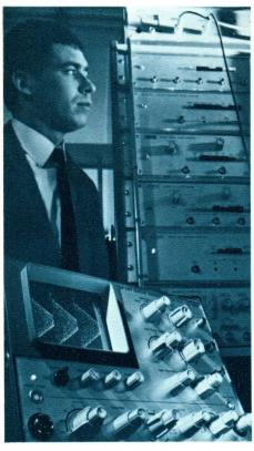
PM 3400; the X-Y output. Shown here is the Philips X-Y recorder PM 8120 making a permanent record of the HF display.
