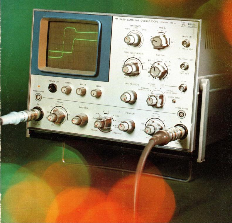
This new Philips 200 ps (1.7. GHz) compact sampling oscilloscope has six special features to make sampling easier, more accurate and more versatile than ever before.
