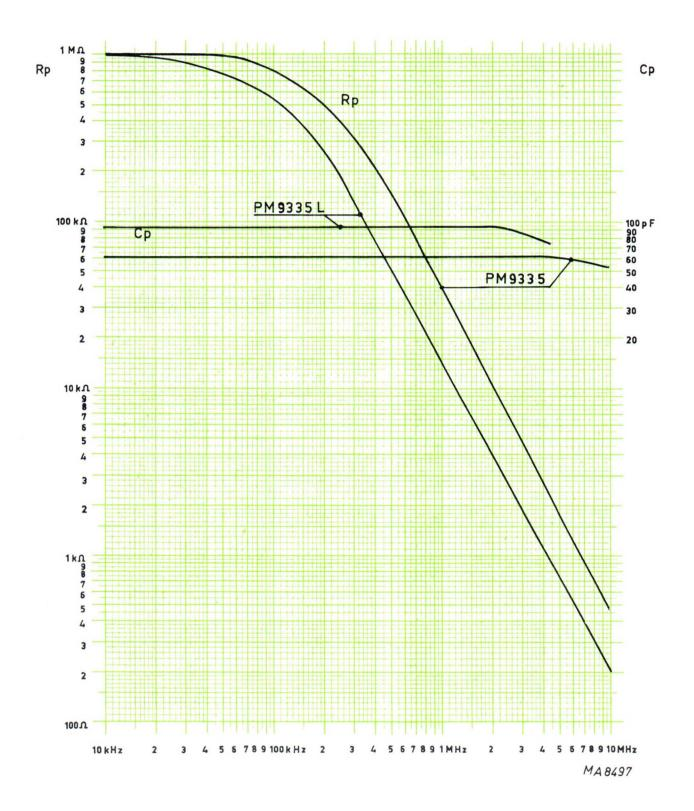
Fig. 1 Parallel input resistance Rp and capacitance Cp as functions of frequency (Probe terminated in 1  $M\Omega//20$  pF)
