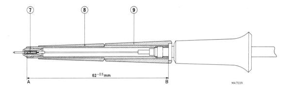
Fig. 3. Cross-section of the probe
