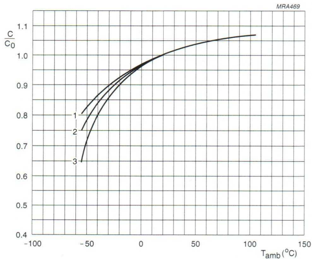
Fig.4 Typical multiplier of capacitance as a function of ambient temperature.
