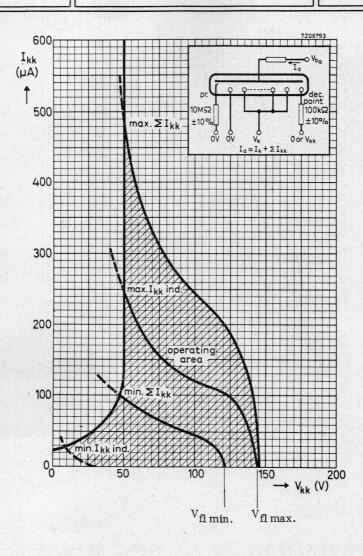
$I_{kk}$  individual and  $\Sigma\,I_{kk}$  versus cathode selecting voltage  $V_{kk}$  at  $I_a$  = 2.5 mA.  $I_{kk}$  and  $\Sigma\,I_{kk}$  are proportional to the anode current within the operating range of  $I_a$  and with  $V_{kk}$  = 0 V to 100 V.
