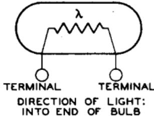
$\lambda$  indicates that the primary characteristic of the element within the envelope symbol is designed to vary under the influence of light.
