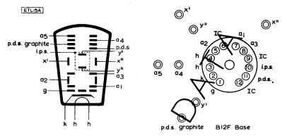
PDS graphite and i.p.s. must be connected together externally
