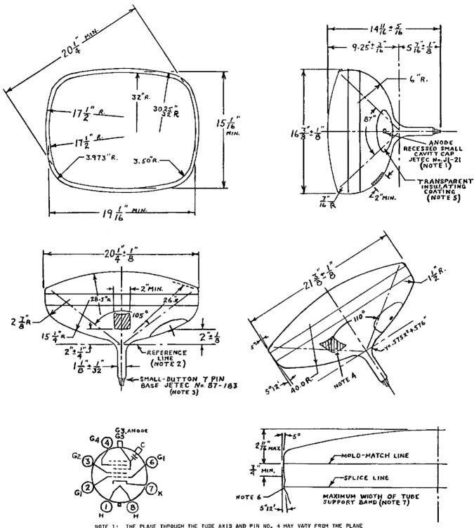
NOTE 1: THE PLANE THROUGH THE TUBE AXIS AND PIN NO. 4 MAY VARY FROM THE PLANE THROUGH THE TUBE AXIS AND ANODE TERMINAL BY ANCULAR TOLERANCE (MEASURED ABOUT THE TUBE AXIS) OF  $\pm~30^{\circ}$ . ANODE TERMINAL IS ON SAME SIDE AS PIN NO. 4.
