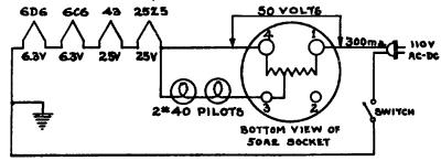
BOTTOM VIEW OF 50B2 SHOWING SOCKET CON-NECTIONS FOR PILOT LIGHT
