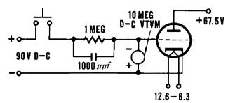
Apply 90 Vdc to grid momentarily. Upon removal of voltage VTVM shall not go positive nor shall it go more negative than -1.5 volts.
